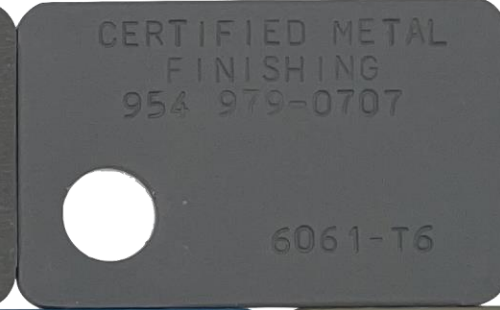
HARDCOAT ANODIZE (TYPE III) THICKNESS 0.002"
